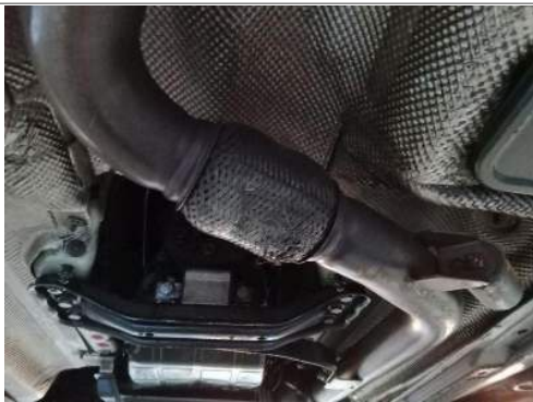
Engine to silencer pipe
