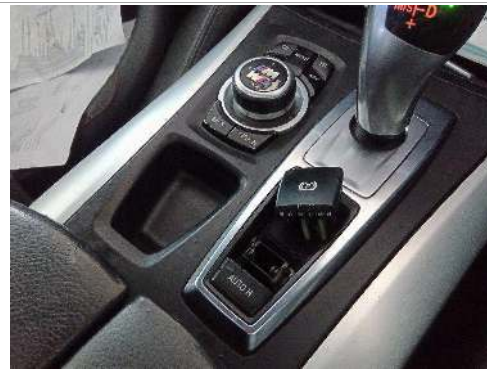
electronic brake switch damage
