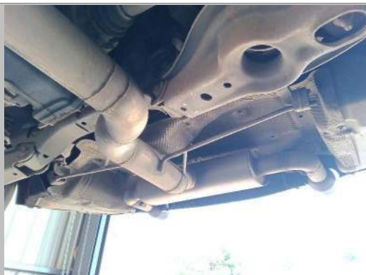
Engine to silencer pipe
