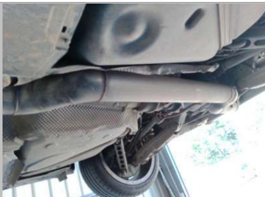
Engine to silencer pipe
