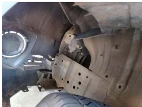
L/F fender liner missing
