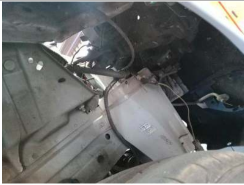
R/F fender liner missing
