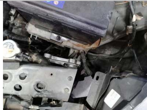
Coolant reservoir missing
