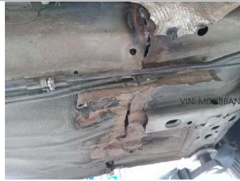
Floor pan cut
