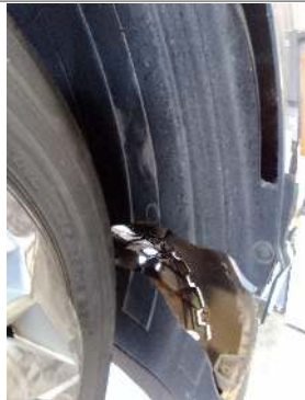
R/F fender liner damage
