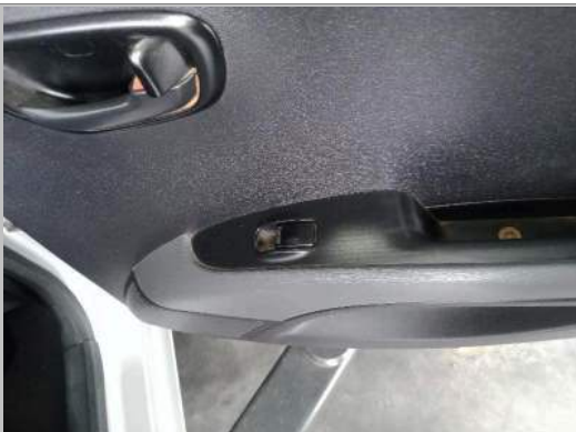
Switch Electrical Window Winder rear right
