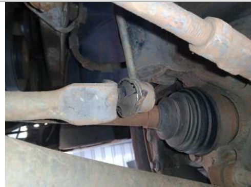
Stabilizer Mounting Front Right
