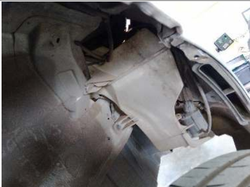
R/F fender liner missing
