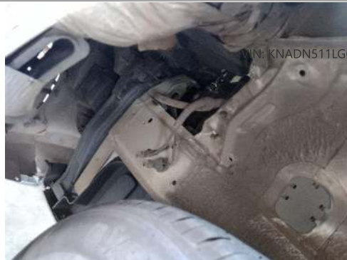
L/F fender liner missing
