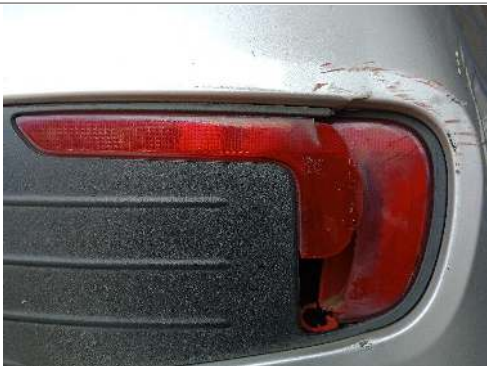
R/R reflector broken
