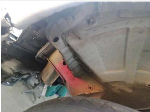
L/F fender liner missing
