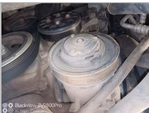
Air conditioner pump
