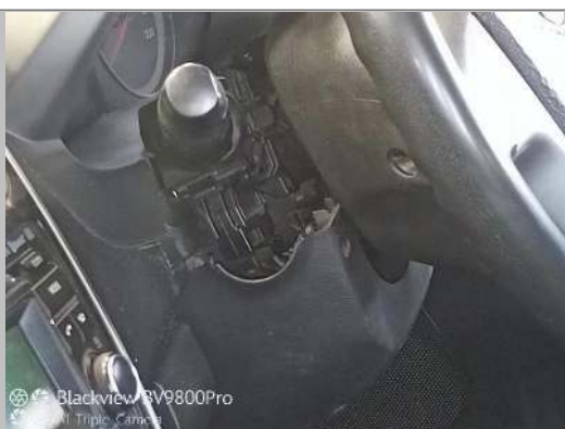
Steering column cover damage
