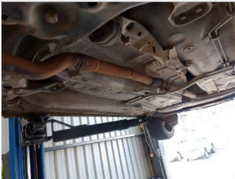
Engine to silencer pipe
