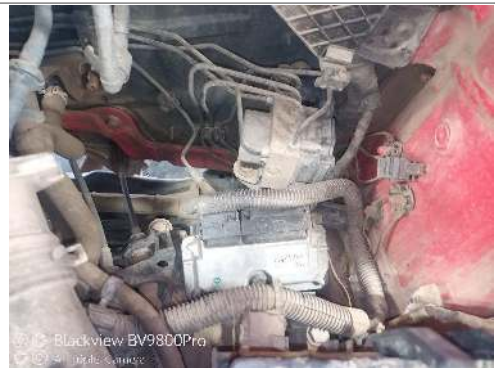
Computer box loose
