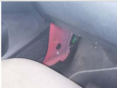
L/F kick panel missing
