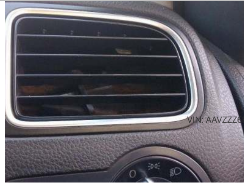
Central Air Vent
