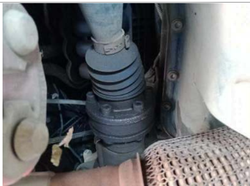
CV Joint(s) Front Right (inner/outer)
